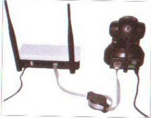
And make sure that the Power indicator light of the router is on (yellow) and the Network Indicator light is flashing (green).
